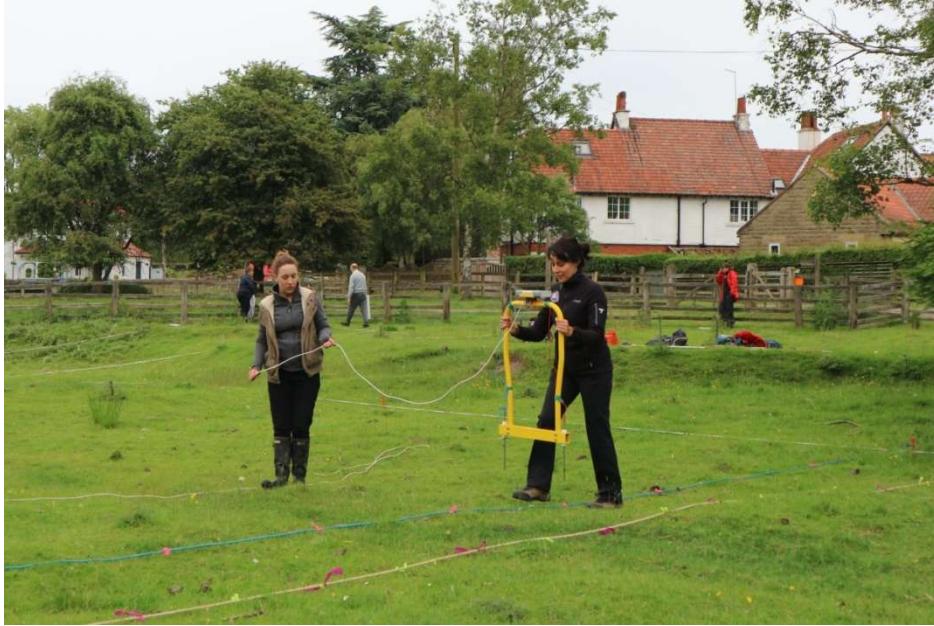
Resistivity meter in use at Goathland, magnetometer in the background
